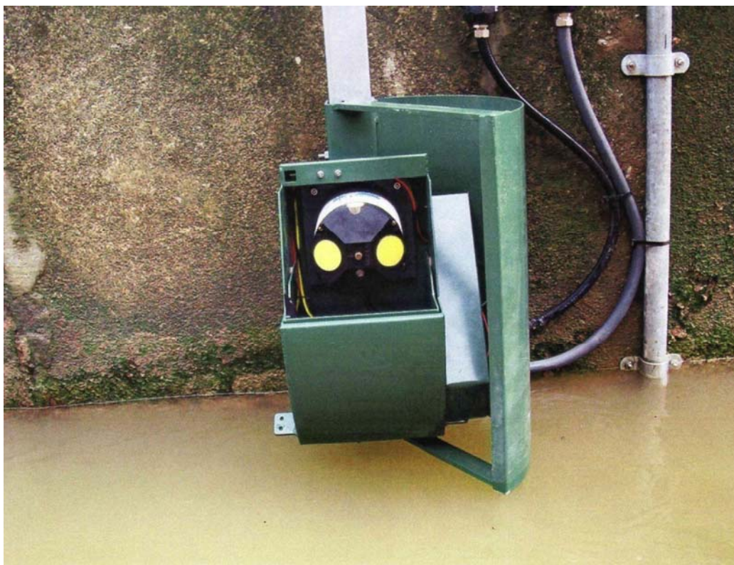
Figure 6: The Doppler Current Meter Provided with a Protective Housing
