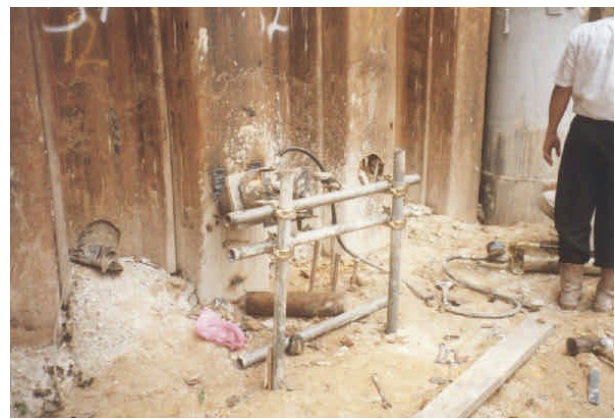
Figure 3 : View of the Pull-Out Test Arrangement
