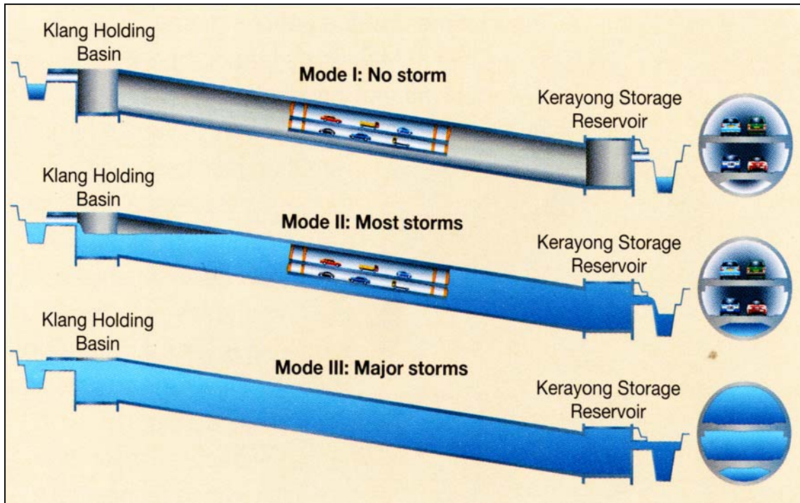
Figure 5: Tunnel Operation Modes
